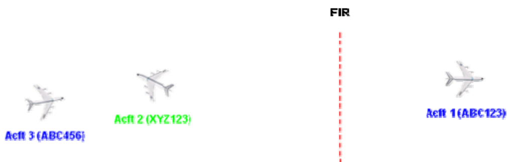
Figure3. As Acft2 was turning back a level request was received from Acft1. This request was misinterpreted as having been made by Acft3. A climb clearance was issued by YBBB to Acft1
