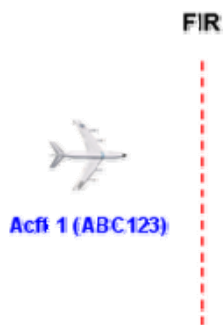
Figure 1. Acft1 does not WILCO the CPDLC transfer instruction approaching the FIR boundary. This resulted in the auto End Service being inhibited.
