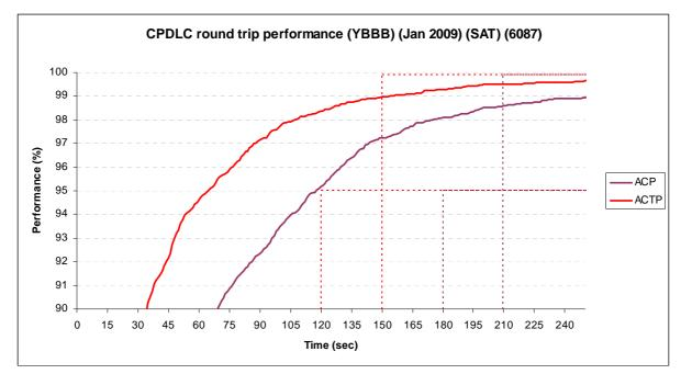
Figure 2 Satellite CPDLC round trip performance
