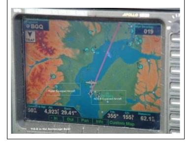
FIS-B transmits graphical National Weather Service products, temporary flight restrictions (TFRs), and special use airspace.
